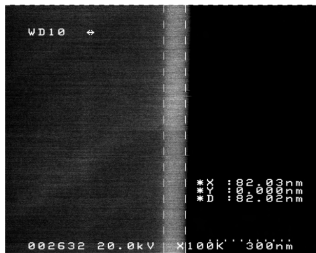
Figure 12. Cross-sectional back-scattered electron (BSE) micrograph of a layer deposited at 600 °C with 6a .
